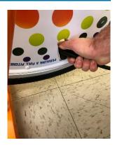
• Pull the lock lever into the closed position. To lock, push lever up away from you.
